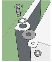
One last Detail – The hinge bolt. The washer arrangement is counterintuitive. If you need to reassemble, place the small washer on the outside, the big washer between the door and the unit. This arrangement allows the door to flex when it is hot.
