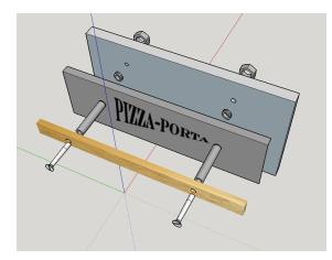
(Hint – push the long screws into the handle and tape over the heads to hold them in the handle. Thread the pieces as shown.)
