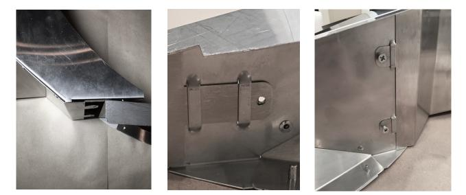
After these three screws are placed in the bales on each side, there is one more screw on the top toward the front on each side that locks in the top panel.
