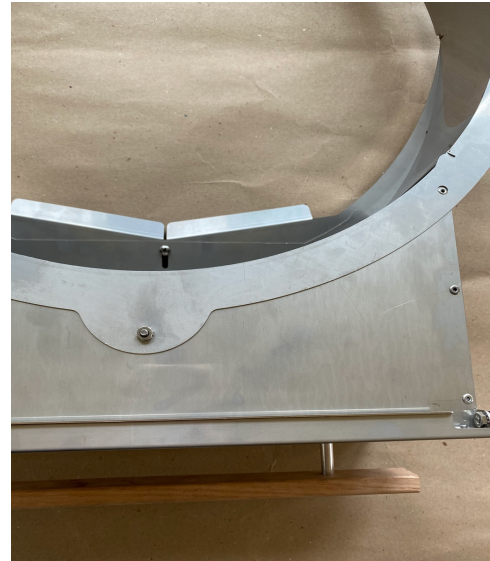
Image 5 – Note clearance holes fit over the bottom ring rivets
