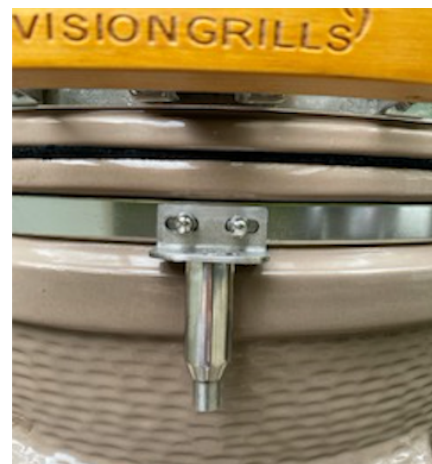
Image 5 – Note clearance holes fit over the bottom ring rivets
